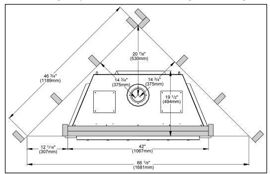
Figure 11. Dimensions for a corner installation.
